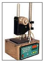
For the tableton system, the coder is mounted on a stand and the item to be printed is placed manually and either a foot switch is pressed or a timer activates to code semi-automatically.
