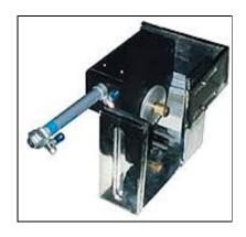
For the on-line system, the print head is mounted on the machine and coding is done whenever the parent machine stops for sealing. It is electronically synchronized with parent machine to give registered coding at exact location.
