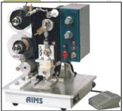
For the tabletop system, the coder is mounted on a stand and the item to be printed is placed manually and either a foot switch is pressed or a timer activates to code semi-automatically.
