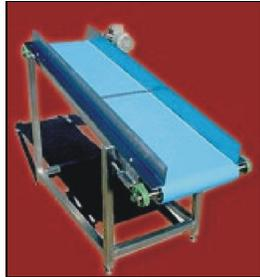
**Continuous / Intermittent Flat Belt Conveyor Model FBC** with polyurethane coated fiber based conveyor belt size 100 mm to 400 mm width X 1000 mm long Stand alone powder coated steel type machine model with 750 mm height. The system has a variable speed setting (pulley based) of 40 / 60 / 80 pouches per minute.
