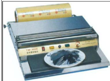
**Tray Wrapping Machine Model -TWM-450** is useful for wrapping transparent cellophane type PVC stretch film on open trays & packets. This type of transparent packing makes the product look attractive as well as increases shelf life.
