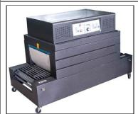
Shrink Packing Tunnel Model SPT-400 where the product is put into the PVC sleeve & passed through the tunnel, the conveyor moves the product through the heat chamber and the finished, sealed product comes out from the other side. These Machines find applications for Stationery, Sweets, Gift Packets, Confectionery, Welding Rods, Bottles, Cosmetics, etc.
